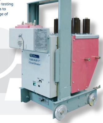
Our VOR-M circuit breaker range has been designed for total reliability. It utilises latest technology ABB vacuum interrupters embedded in resin for high dielectric performance and protection against shock, humidity and dust. For ultra reliable performance we have incorporated a magnetic actuator drive which reduces the number of moving parts to the absolute minimum to achieve trouble free performance over many thousands of maintenance free operations.
