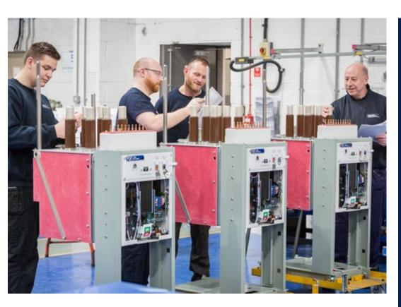
Typically: 12kV, 400A, 630A, 800A, 1250A and 2000A with 20kA, 25kA, and 40kA fault rating options, 75kV BIL
